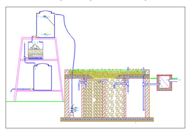
Figure 2-4 Illustration of onsite grey water treatment plant (Burnat and shtayye, 2009)
